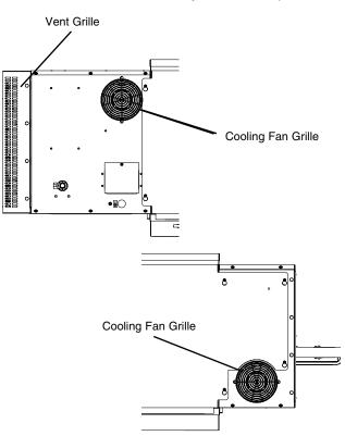
Figure 4-1. Oven Cooling Fans
